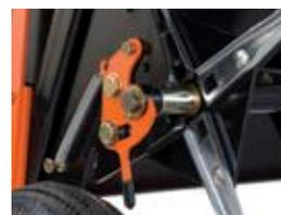
SmartLINK™ system patented locking device enables attachments to lock in and unlock in seconds.
