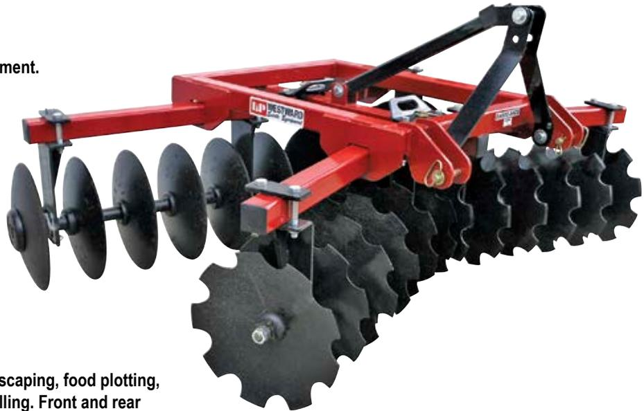
The Disc Harrow is an ideal choice for landscaping, food plotting, gardening, small acreage or general farm tilling. Front and rear gangs are easy to adjust with our built-in adjustment handle. The 7 1/2" disc blade spacing allows the blade to cut evenly over the ground. The 3" square tubing is heavy enough to pull an attachment behind the disc harrow to better level the soil.
