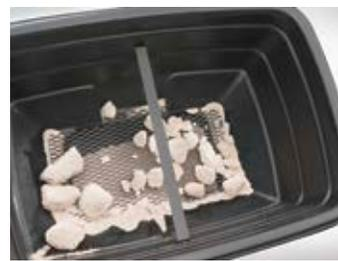
Agri-Fab® UTV/ATV compatible spreaders include a spreader grate which improves material flow and performance.
