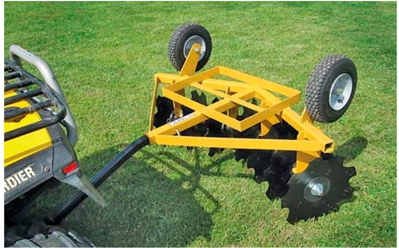
*Flip-over disc incorporates a square weight frame in its design which allows the operator to strap 3 concrete blocks to the top of the disc, increasing its weight for more aggressive soil penetration.*
