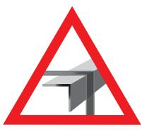
Global Sharp Edge symbol– Radius as sharp as .005 in. (.13mm)
