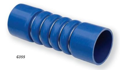
In some applications where the distance between the engine and radiator connection is very short, the vibration and movement will cause premature failure of standard coolant hoses. G355 connectors (often known as hump hoses) feature corrugated sections supported by steel rings that allow for much greater flexing than a standard hose.
