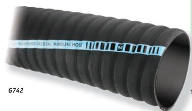
Groundhog Hose is a lightweight hose used for suction of sand, soil and a variety of other abrasive materials. Its flexible design makes it ideal for truck mounted hydrovac service for drain cleaning, daylighting, and other waste cleanup.
