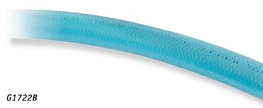
G1722B is an example of the breed of new polyurethane hoses. This hose is amazingly tough and puncture resistant, yet it weighs less than PVC hoses, and much less than rubber. The polyurethane compound is formulated to stay flexible down to -40°C, and it has excellent resistance to oils and solvents.
