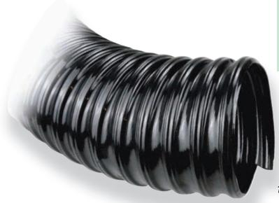
In our most popular sizes, we offer our Thermoplastic Urethane Ducting with a lighter 35 mil wall thickness. While maintaining the excellent wear resistance properties of urethane, TPU35 offers a more competitively priced alternative for customers with less demanding applications such as chemical fume removal, powder transfer, and seeding.
