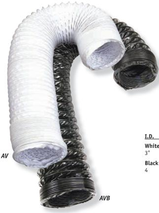
AV is a lightweight vinyl duct supported by a steel wire for use in venting bilge fumes. It is also suitable for bathroom fan and general purpose air exhaust. In the past, AV was commonly used for venting clothes dryers, however it is no longer recommended for that application. Clothes dryer duct should be UL listed and be made from a metallic fire resistant material.
