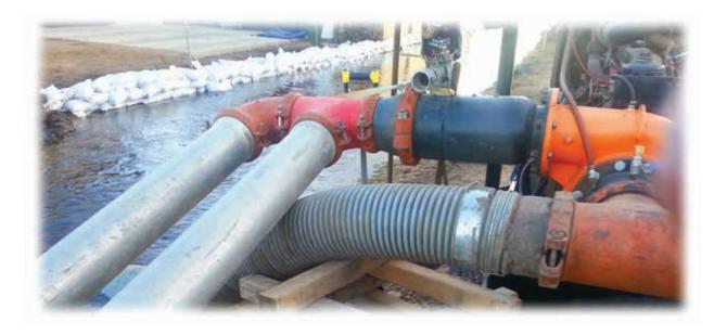
G941WS incorporates a polyester fabric braid for applications requiring a greater working pressure than suction hoses reinforced with a spiral helix only.
