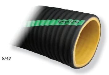
Rhino Hose is our heaviest hose and is ideal for handling slurries, gravel, ore, groundfish, and other abrasive materials where conditions are severe. The corrugated cover is designed to fit an over-the-cover flange fitting system. Flanges feature corrugated coupling sleeves that fit tightly over the hose when flange halves are bolted together. This provides a full-flow coupling that can be installed in the field.
