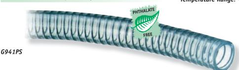
Working Vacuum Min. Pressure Bend Weight Standard Part Rating I.D. Number 0.D. 20°C 50°C 20°C Radius per ft Length 1/4" G941PS-025 0.45" 1" 150 psi 70 psi 29" Hq 0.07 lb 100 ft 3/8 G941PS-038 100 70 1.5 0.60 29 0.11 100 See 1/2 G941PS-050 100 70 29 2 100 0.74 0.15 Prices Online 5/8 G941PS-063 0.86 100 50 29 100 2.5 0.18 3/4 G941PS-075 1.03 70 50 29 0.25 100 3 1 G941PS-100 1.29 70 35 29 4 0.32 100
