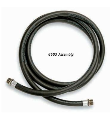
Since farm tank is most often sold in short lengths coupled with male pipe fittings, we offer these assemblies already made up. Our 3/4" and 1" farm tank hoses feature brass plated zinc fittings attached with crimped aluminum ferrules. The 11/4" hoses have aluminum ends attached with band clamps. Internal spring guards in each end of all 3/4" and 1" hoses prevent kinking next to the fittings.
