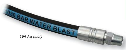
Water Blast hose is often found in hydro-demolition (concrete breaking using water instead of a jackhammer). It is also used for cleaning large tanks, heat exchangers and pipes, as well as for removing marine growth on ships and piers. Since only water is used in the work, rather than chemicals or abrasives, water jetting is an environmentally friendly method of cleaning and surface preparation.
