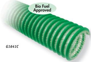
G1641C is different from other PVC gasoline drop hoses currently found in the market. It has a unique polyurethane tube that combines the advantages of good chemical resistance, light weight, and low temperature flexibility. G1641C is now green to signify that it is suitable for use with ethanol (up to E98) and biodiesel fuels that conform to ASTM D6751 (up to B100). This product comes complete with a static wire to ensure positive grounding when properly coupled.
